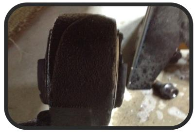
Lubricate bushing with soapy water and begin tightening nut to draw bushing into housing. Be sure bushing is being drawn in evenly. Stop drawing bushing through once exposed portion of bushing is even on both sides of the housing. Bushing installation is now complete
