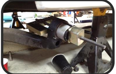
Install bushing tool on subframe with U-Shaped block seated against inner face of trailing arm. Slip new bushing over threaded rod. Slip rectangular washer over threaded rod and seat against new bushing. Thread threaded block down the rod until snug against rectangular washer (see photo).
