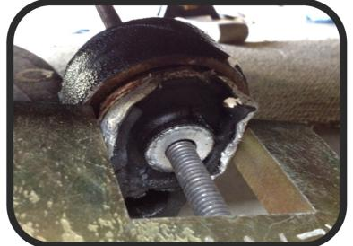
Begin tightening nut. If excessive force is required, be sure tool components are properly seated against their respective parts. Try a penetrating fluid to loosen corroded bushings and housings.
