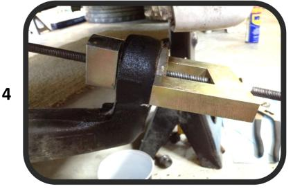
Install bushing tool on trailing arm. Set aside rectangular washer—this part will only be used when installing new bushing. Thread the threaded block over the threaded rod bored-out portion first (to fit over metal portion of bushing).
