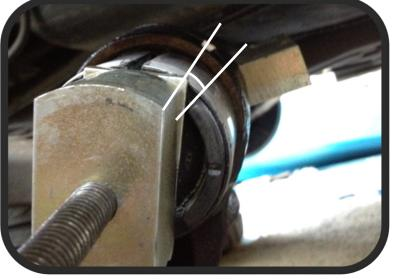
Align new bushing with reference mark made in step 3. Turn the bushing about an 1/8" away from the reference mark in the clockwise direction (looking at the outer side of the trailing arm). The action of tightening the nut will often rotate the bushing in the clockwise direction, bringing bushing into proper alignment.
