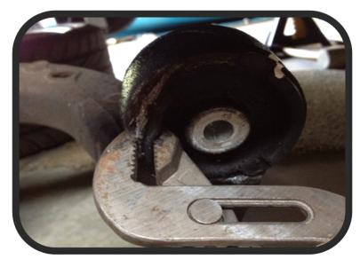
Unbolt bracket from bushing and remove from trailing arm. Use a utility knife to cut excess bushing material from the inside of the bushing. Older bushings have metal ring surrounding entire bushing... bend metal edges around outer rim of outer face of bushing so that the tool will be able to seat against the trailing arm (see photo) - Newer bushings have two slots cut out of metal ring so that bending is not required.
