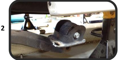
Use paint pen to mark orientation of forward trailing arm carrier bracket for later re-installation.
