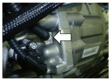
Note the location of the potentially loose cannon ground connection on the engine block near the starter.
