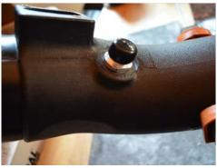
15. If not equipped with crank case line. Cap the crank case fitting with the 3/4" vinyl cap
