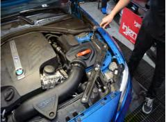
18. *IF EQUIPPED*: Reinstall the strut tower brace.
