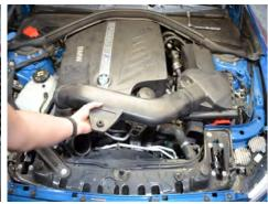
6. Remove the OEM intake assembly.
