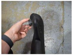
10. Install the grommet into the Injen tube.
