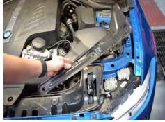
5. IF EQUIPPED: Remove the strut tower brace.
