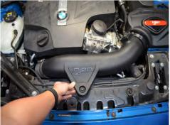
13. Press the injen tube into the turbo inlet pipe. Next 14. Connect the MAF harness. press the tube into the twist lock filter. Finally line up the *IF EQUIPPED*: Connect the crank case line.
