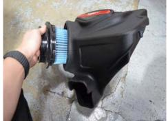
11. Install the twist lock filter on to the Injen air 12. Install the Injen air box into the engine bay. box. Once seated, rotate the filter a 1/4 turn in either direction so the filter can lock into place.
