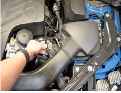
2. Disconnect the MAF harness. IF EQUIPPED: Disconnect the crank case line.
