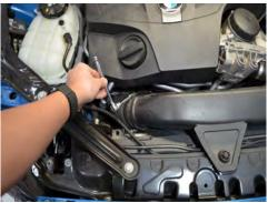
3. Loosen the clamp holding the OEM tube.
