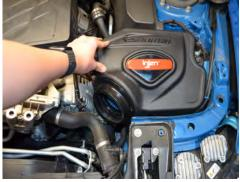
Line up the studs on the air box to the factory grommets and press down on the box.
