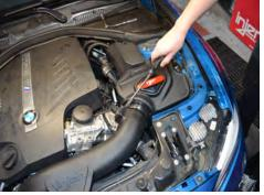
17. Secure the clamp on the twist lock filter.
