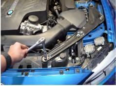
4. IF EQUIPPED: Remove the four bolts holding the strut tower brace.
