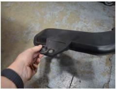
9. Remove the grommet from the OEM tube.
