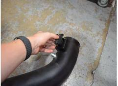
8. Install the MAF sensor into the Injen tube and secure using the provided M4 x 0.7 button head screws.
