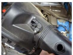
7. Remove the two screws holding the MAF sensor and then remove the MAF sensor.
