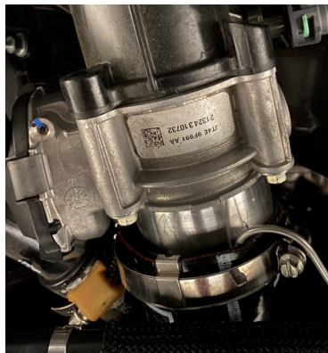
BEST (INTAKE HOSE AT ENGINE THROTTLE BODY)
