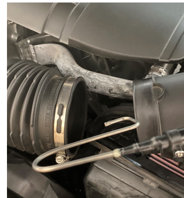
ACCEPTABLE (INTAKE NEAR ENGINE THROTTLE BODY-ONE INTAKE HOSE BEND)
