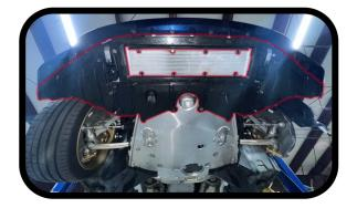
Remove the Lower engine covers and oil cooler shroud.
