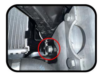
Next the aux cooler through bolts gets installed, torque the two bolts here to 50nm (37 ft $\bullet$ lbs) .
