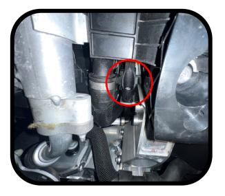
Reattach the oil cooler bracket.
