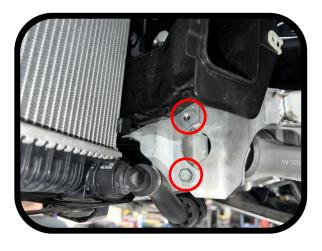
Getting the bracket back in place can be a little tricky. Pull the aux cooler line out of the way and work the box back and forth until it slips up far enough to get a bolt through the lower hole.
