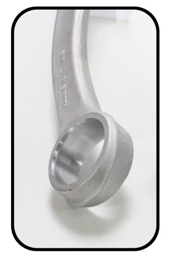
Remove the factory bushing from the tension strut by cutting or pressing out the bushing.
