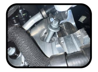
Reinstall the tension strut using the included replacement nut and bolt. Torque the subframe bolt to 68Nm + 180 Degrees.
