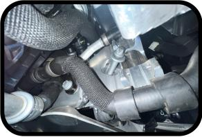
With the bracket removed you will now be able to access the bolt holding in the tension strut.
