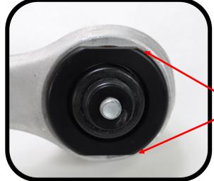
The housing is installed in two halves, the ball joint housing is pressed into the tension strut and secured with the cap and screws.
