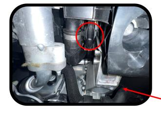
On the inside of the bracket there is a screw holding on the oil cooler bracket. You will need a long extension to reach this.
