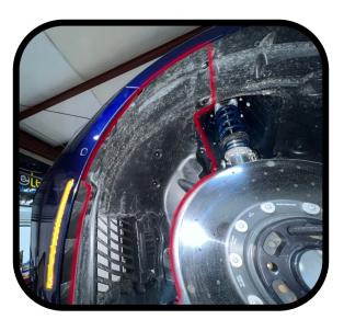
Reattach the lower engine covers and the inner fender liner.
