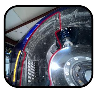
Start by removing the front wheels and inner fender liners.
