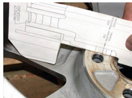
6. Verify that the edge of the caliper does not touch the rim or the wheel spokes. A minimum clearance of 2mm (0.080") is recommended.
